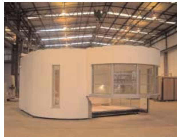
Main picture and above: Atelier One created a prefab penthouse that was craned onto the art deco Thompson House, Cheshire.
